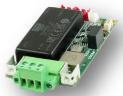
PW505 Isolation power board with CPC-Ignition on/off control 1.5KVDC I/O isolation PW505-36: 9-36V in, 12V out, max 60W PW505-75: 18-75V in, 12V out, max 60W
