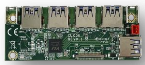
CU006 1 x USB convert to 4 x USB 3.0 HUB
