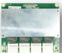
CU006 1 x USB convert to 4 x USB 3.0 HUB
