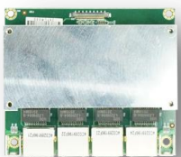
CU006 1 x USB convert to 4 x USB 3.0 HUB
